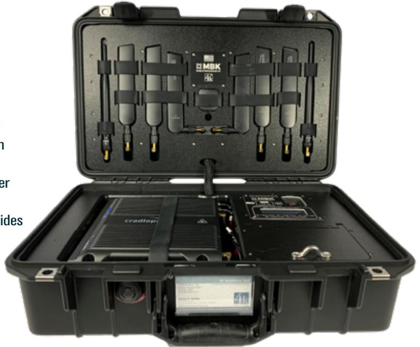
**MBK™ 1700 FI** a 4G/LTE solution that contains the CradlePoint IBR1700, ClearRF amplifier and integrated LifePo4 battery.
