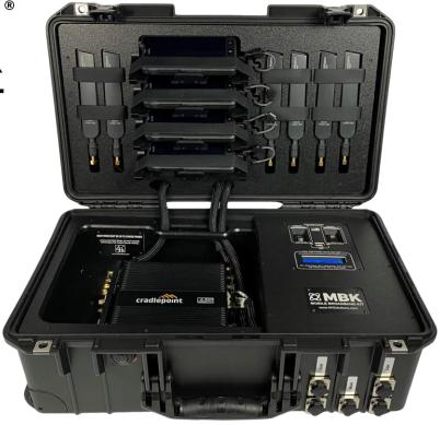
modems support worldwide, SIM-based, auto-carrier selection and also available CBRS Band 48 and a Band14 FirstNet<sup>™</sup> Ready MC400 modem. The **MBK Elite XP8** provides 802.11 wireless and ethernet networking options.
